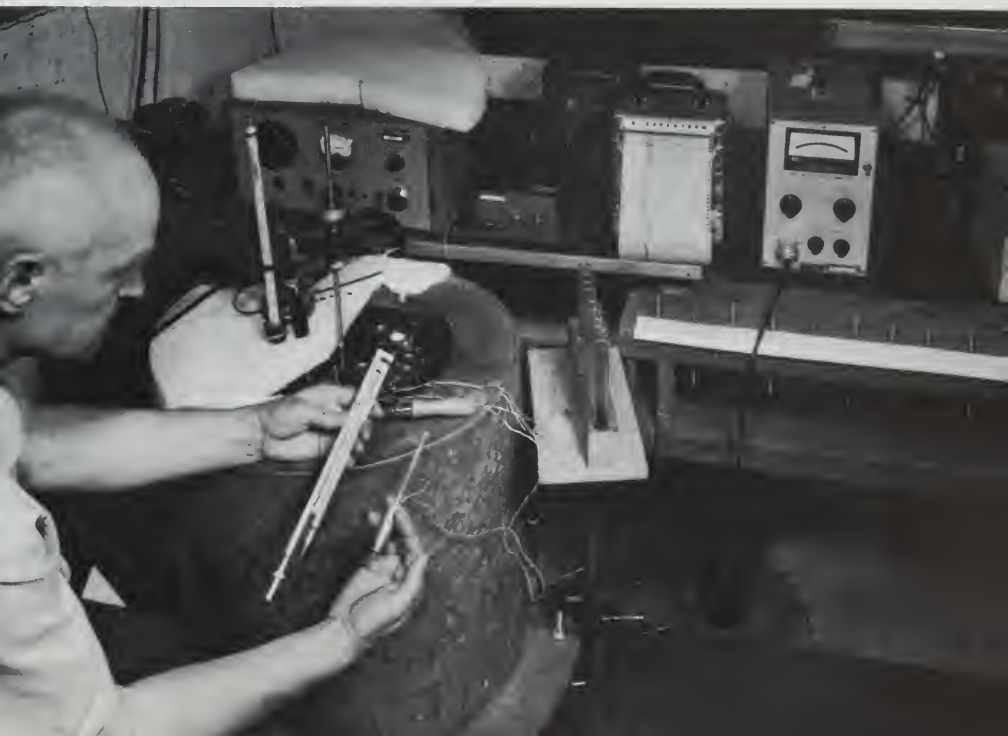
Dr. L. A. Richards of the Salinity Laboratory uses psychrometers to measure the relative humidity of water in soil.
